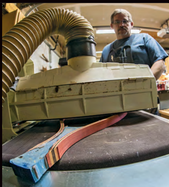
An overhead drum sander is used to sand down net hoop laminations of Bolivian redheart, Honduran mahogany, and African wenge so they are flush with the net's handle.
