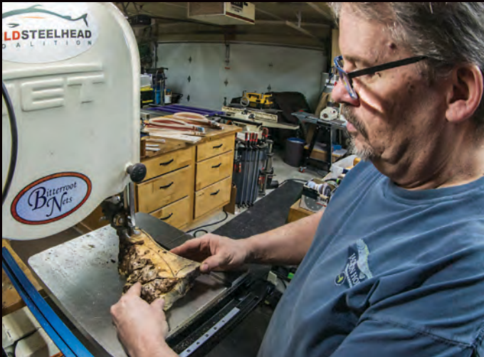
The handle for a Stream Net is carefully cut from an intricately figured section of buckeye burl. Mostly found in California, buckeye burl is a root ball burl that is prized for its multicolored chatoyance.
