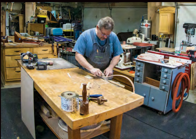
After multiple machining steps to build a net, Carson applies the final shaping and sanding by hand, and then begins his nine-step waterproofing finish process.
