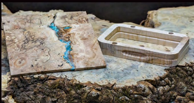
The frames of Bitterroot fly boxes are fastened together with lock miter joints. This box and lid will become one of the River Series boxes.
