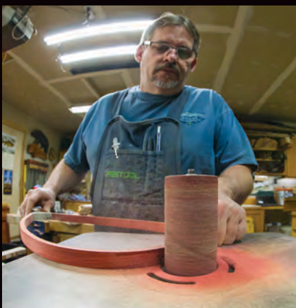
Denny Carson, founder of Bitterroot Nets, carefully sands the hoop of one of his nets in preparation for the installation of the magnetic carry system, or I-MAG.
